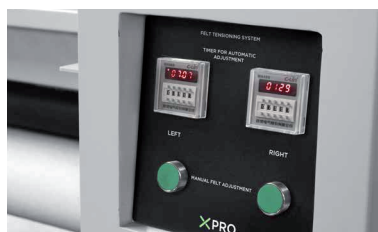
Felt belt automatic tracking system
