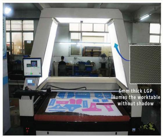
7. The camera on the top of machine captures all patterns on the worktable one time, then with the help of applicable software, the patterns photo will be input into the computer and after DSP processing it, the machine will locate the pattern edge, thus the laser head will cut materials along the edge of patterns.
